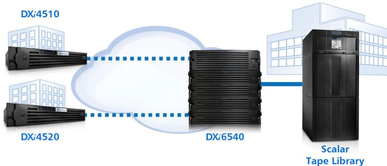
*The DXi4500 protects remote sites with disk, provides automated DR protection using replication, and enables tape consolidation.*
